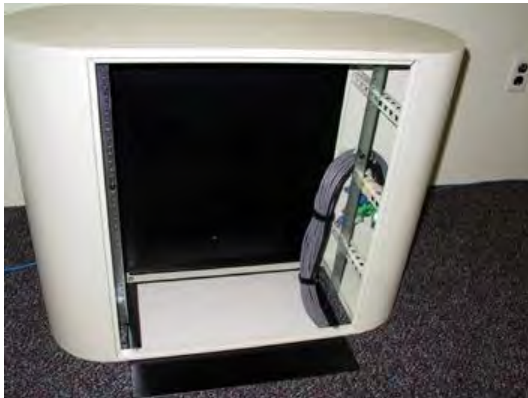
LDS with Data Cables fed through base
