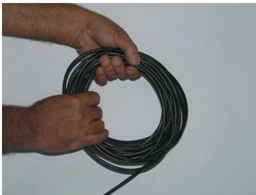
Correct !!! Hand over hand unrolling out.
