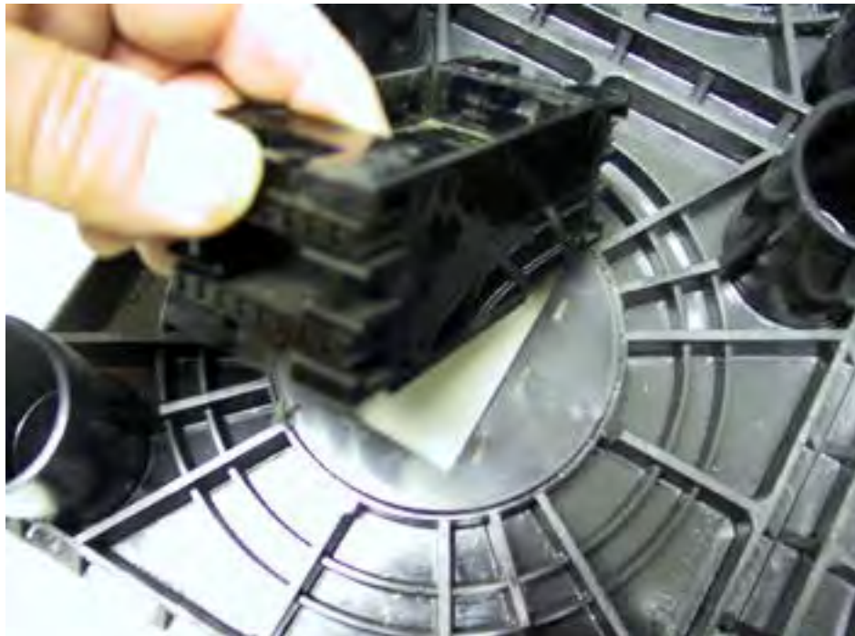
Picture 9-8 Installing Powerport Clips
